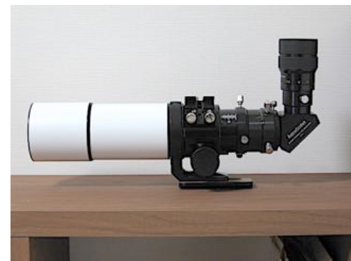
BLANCA-60SED 31.7mm 天頂ミラー with 2inch 35mm-extension tube & 7.2mm - 21.6mm zoom eyepiece
